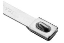
316 grade stainless steel offers excellent resistance to salt spray, corrosion, weather and chemical resistance.Self locking, ball bearing mechanism for quick and easy installation, either by hand or by tensioning tool.
