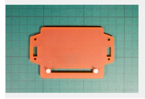
Push the two M2.5 bolts through the frosted orange layer and then screw two of the nuts on tight (these are the spacers). Now, slide your Scroll pHAT HD down onto the bolts, so that the LEDs are facing towards the acrylic. Use the remaining two nuts to secure the pHAT.
