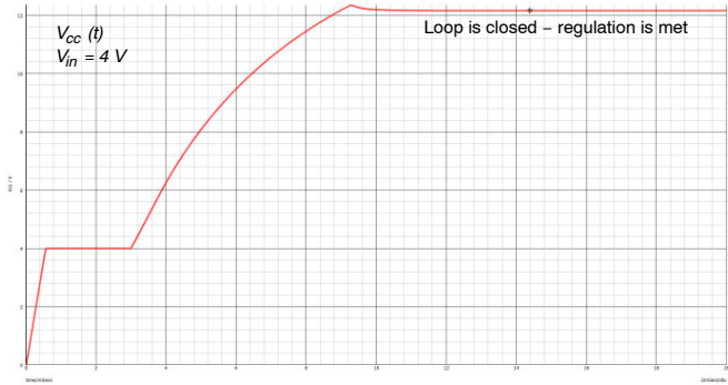
Figure 35. The LDO Can Be Associated with an Auxiliary Winding and Be Turned Off in Normal Operation
