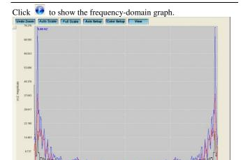
The software computes real-time spectral data using an FFT from 0 to 256 HZ.
