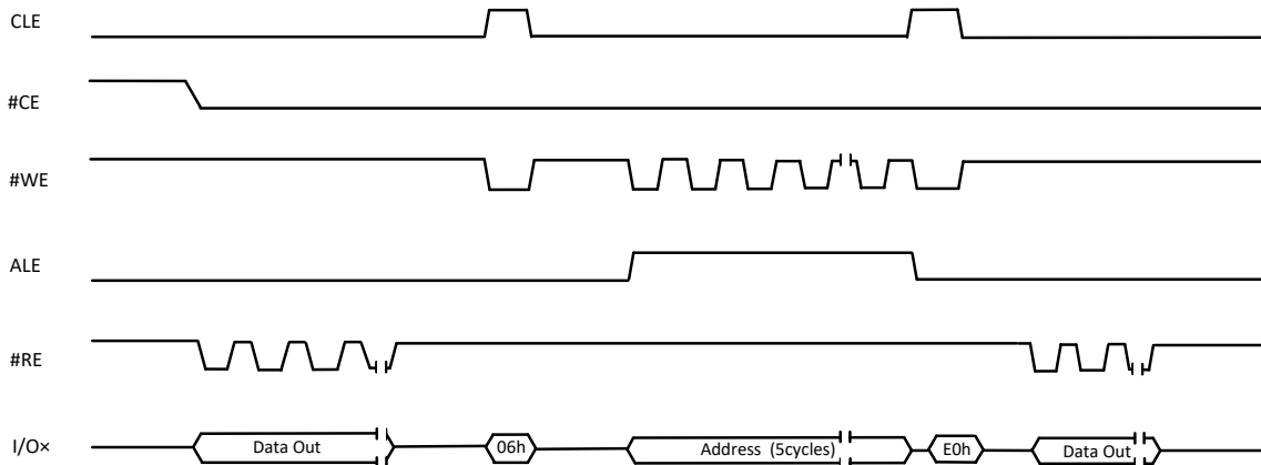
Figure 9-4 Two Plane Random Data Read (06h-E0h) Operation
