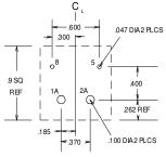
MOUNTING HOLE PATTERN TOP OF PCB
