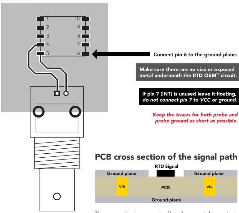
This cross section is an example of how the ground plane protects the RTD signal. The ground plane should surround the RTD signal, on the top layer as well as the bottom layer.
