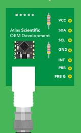
Do not solder wires to this device.
