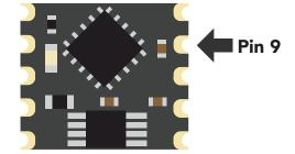
The Interrupt control register adjusts the function of pin 9 (the interrupt output pin).
