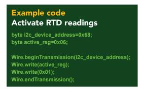
Once the device has been woken up it will continuously take readings every 420ms. Waking the device is the only way to take a reading. Hibernating the device is the only way to stop taking readings.
