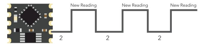
The pin will not auto reset. 2 must be written to the interrupt control register after each transition from low to high.
