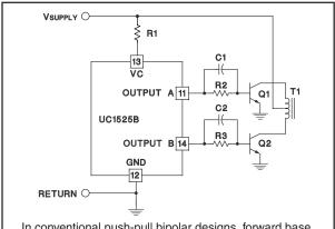
In conventional push-pull bipolar designs, forward base drive is controlled by R1-R3. Rapid turn-off times for the power devices are acheived with speed-up capacitors C, and C2.
