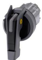
Illuminable selector switch, 22 mm, round, collar, metal front ring, metal matte, black, Selector switch long, 3 switch positions I-O-II, latching, actuating angle 2x45°, 10:30h/12h/13:30h, can be locked in I + O, with 2 padlocks, or snap hook, shackle 5 mm, can be combined with metal holder
