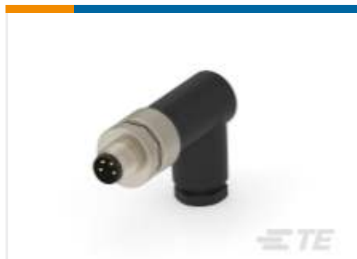
TE Part #T4013008041-000 M8,SCREW, MALE,R/A,UNSHIELD,4P, GOLD
