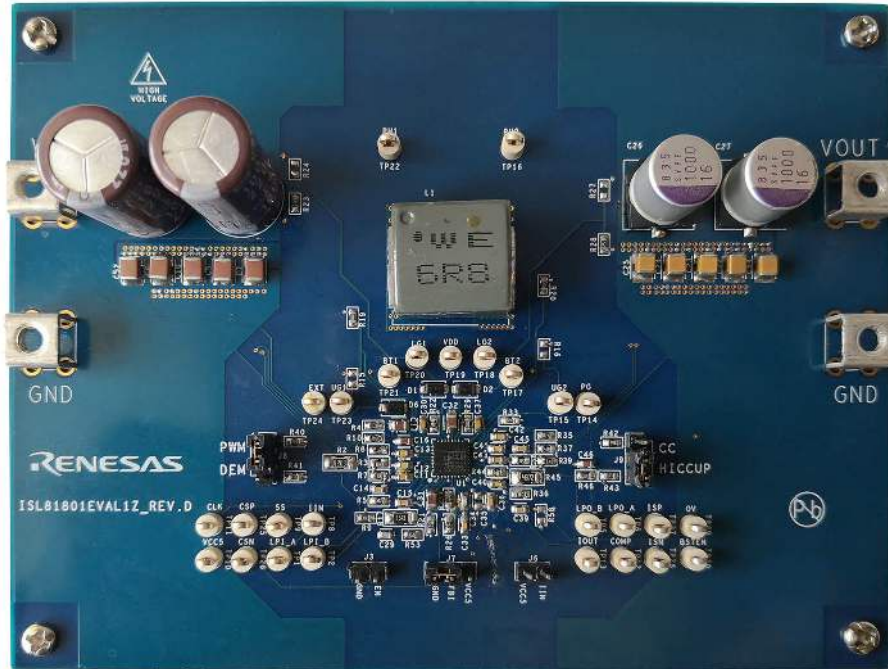
Figure 5. ISL81801EVAL1Z Evaluation Board, Top View
