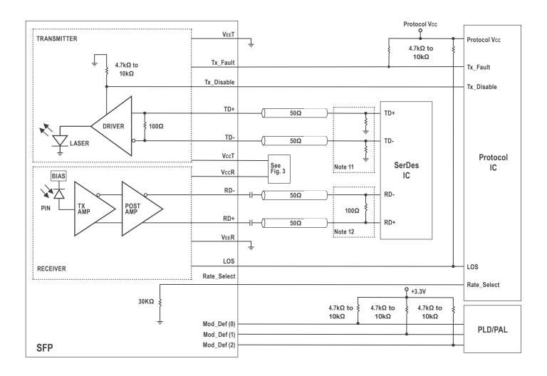
Figure 1 Illustrates the recommended transmit and receive data line terminations.
