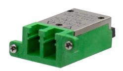
The FNK-ER12x singlemode optical fiber transceivers provide low profile, cost effective solutions for Gigabit Ethernet and 1x Fiber Channel optical fiber data links, up to 55 km distance using 0.25 dB/km singlemode cable, with a duplex LC connector interface. These transceivers are fully compliant with the IEEE Gigabit Ethernet and ANSI 1x Fiber Channel standards but can be used for any other data communications purpose within their operating parameters.
