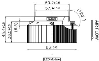
Assembly direction of customer's LED Module
