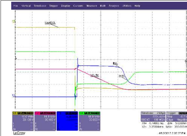
V_{IN,A} = 54\text{ V} ; V_{IN,B} = 38\text{ V} , scope GND = RTN, Iload = 5 A
