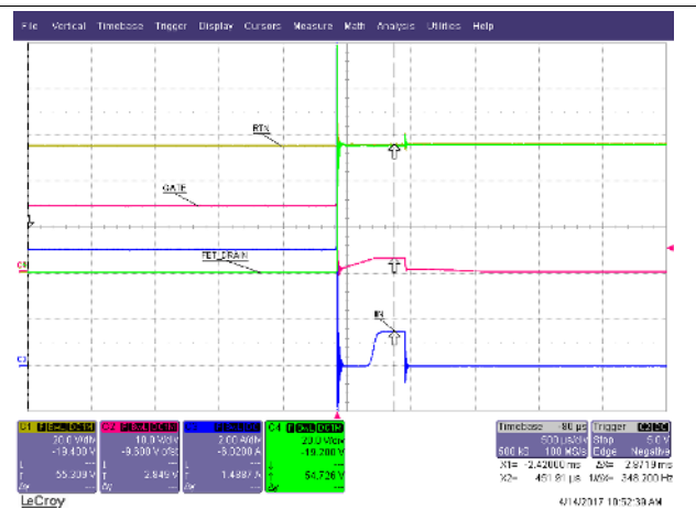
Scope GND = -48V_B, 5-A load, after inductor
