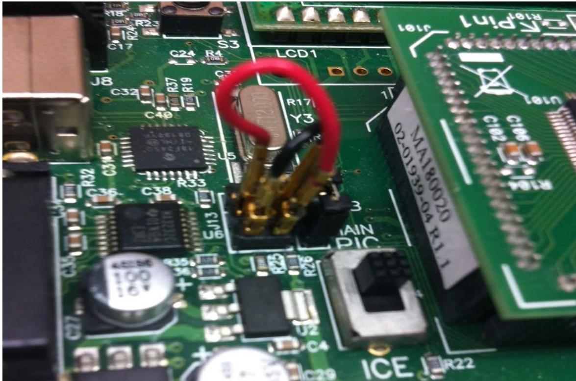
Figure 2. Jumper Selection for Command Mode Operation
