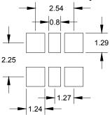
Note: XPRESSO LVDS XOs are designed to fit on Industry standard, 6 pad, layouts.
