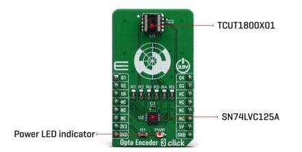
Since the signals of these output channels are not enough to drive pins on a host MCU, the Click board<sup>™</sup> features two additional buffer IC – the SN74LVC125A, from texas instruments. E1, E2, E3, and E4 pins are routed to the input pins od the buffer IC. These pins are pulled to a LOW logic level by the pull-down resistors, to avoid floating.
