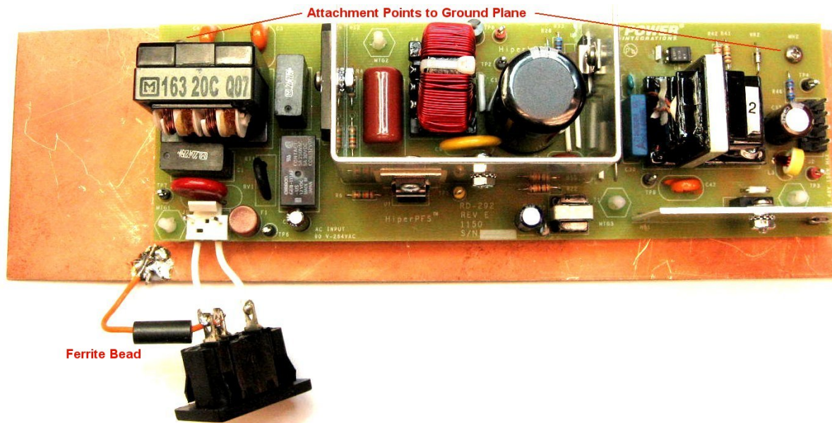
Figure 78 – RD-292 Set-up for EMI and Surge Testing.
