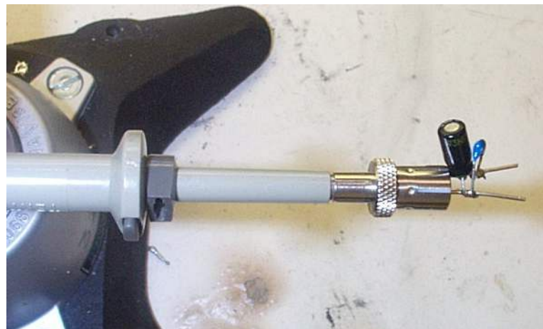
Figure 40 – Oscilloscope Probe with Probe Master 4987BA BNC Adapter (Modified with Wires for Probe Ground for Ripple measurement and Two Parallel Decoupling Capacitors Added).
