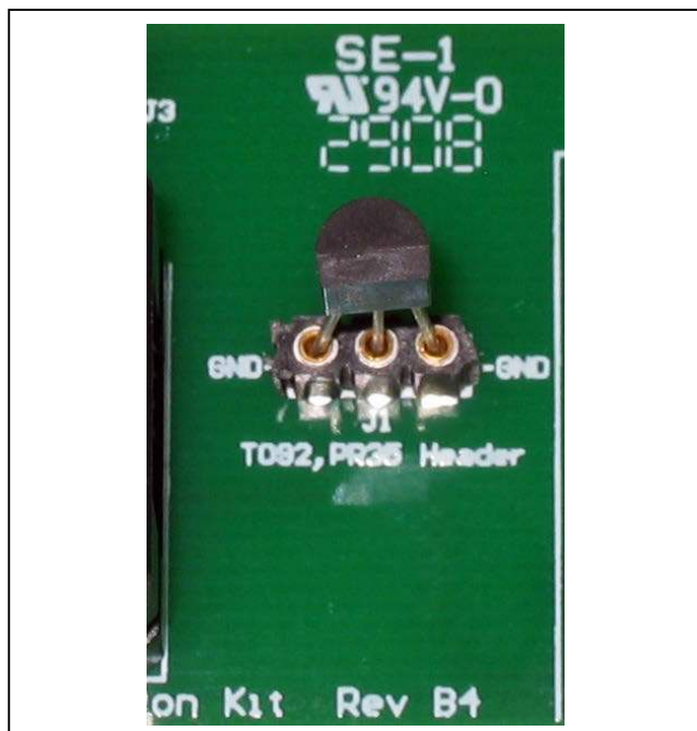
Figure 3. TO92/PR35 Package Insertion
