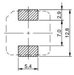
no sensitive traces underneath the component
