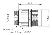
Main Dimensions Receptacle \*for max. wire cross-section pay attention to the cross-section of used contacts
