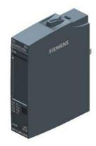
SIMATIC ET 200SP, Digital output module, DQ 8x 24V DC/0,5A Basic, Source output (PNP,P-switching) Packing unit: 1 piece, fits to BU-type A0, Colour Code CC02, substitute value output, module diagnostics for: supply voltage
