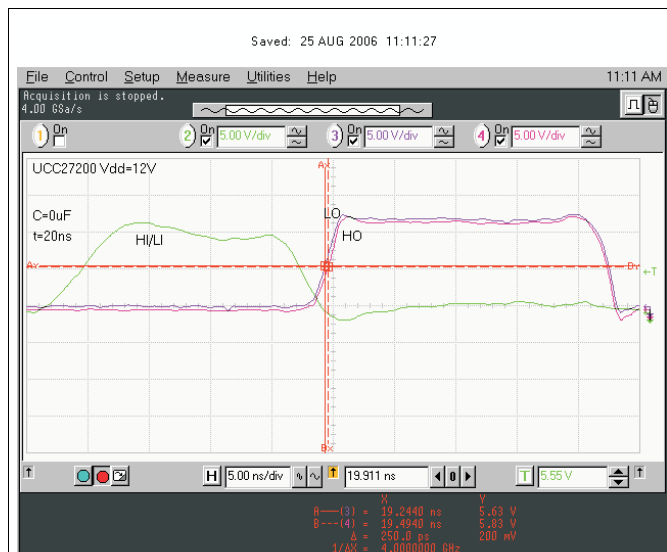
Figure 32. 20-ns Input Pulse Delay Matching
