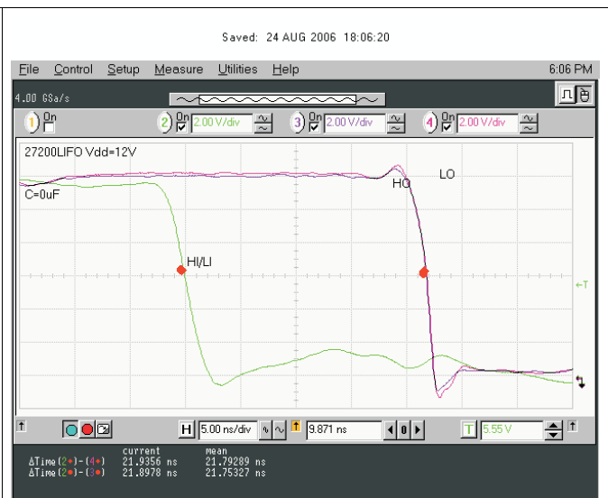
Figure 31. V_{LO} and V_{HO} Falling Edge Delay Matching
