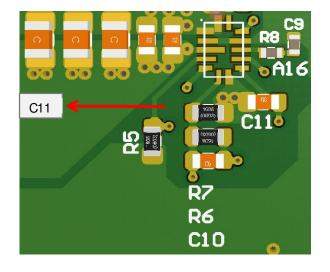
SS time is set at default of 1.4 msec. Adding a small MLCC capacitor between REF and RTN can extend the soft start time.
