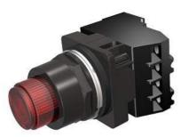
30mm BlackMax, Epoxy Coated Corrosion Resistant Complete Metal Unit PTT / Illuminated Pushbutton Full Voltage, 12V AC/DC Incandescent Lamp Extended Button Plastic Lens, Red 2 Position Momentary with 1 N.O. - 1 N.C. Heavy Duty Contacts, A600/P600 UL Listed, CSA Certified NEMA 1,3,3R,4,4X,12,13 & Automotive Standards
