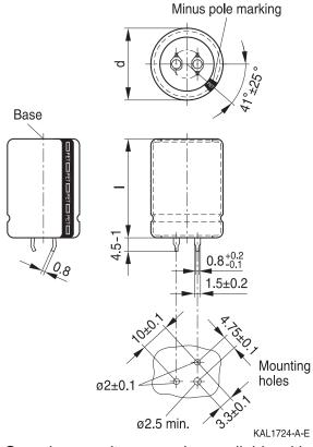
Snap-in capacitors are also available with 3 terminals (length (4.5-1) mm). Insulation is marked with "PET" on the sleeve. Safety vent on the case wall.
