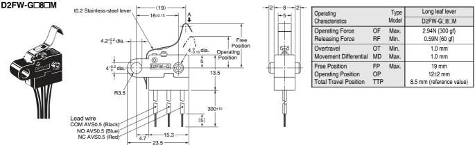
Note1. Unless otherwise specified, a tolerance of ±0.4 mm applies to all dimensions. Note2. The operating characteristics are for operation in the A direction (  $\clubsuit$  ).
