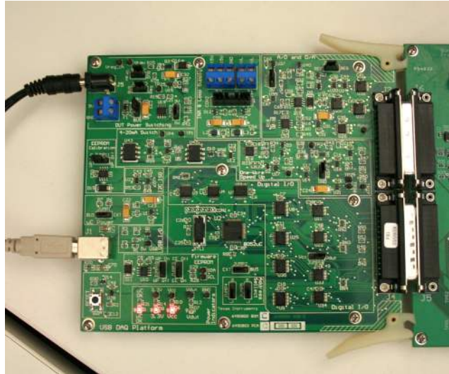
Figure 10. Connecting the USB Cable to the USB DAQ Platform
