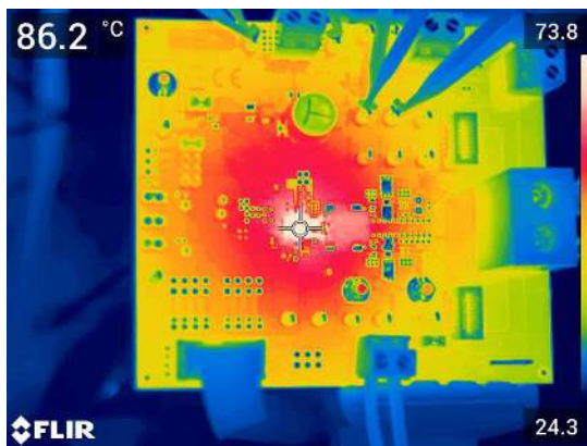
Figure 8-21. Thermal Characteristics, 600 kHz FCCM, Internal LDO, 35-A Load
