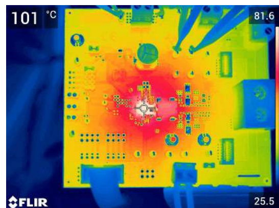
Figure 8-26. Thermal Characteristics, 1.2-MHz FCCM, External 5-V Bias, 35-A Load
