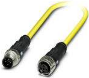
Sensor/Actuator cable, 4-position, TPE, yellow RAL 1021, Plug straight M12 SPEEDCON, A-coded, on Socket straight M12 SPEEDCON, A-coded, Cable length: 1.5 m
