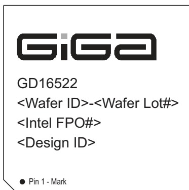
Figure 11. Device Marking. Top View.
