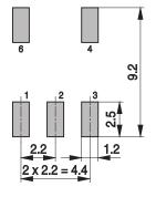
Recommended PCB layout (top view)
