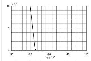
Fig.24. Typical negative load clamping.  $I_L = f(V_{LG})$ ; conditions  $V_{IG} = 0V$ ,  $T_j = 25^{\circ}C$
