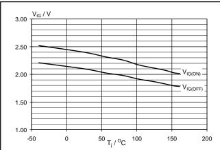
Fig.17. Typical threshold voltage characteristic.  $V_{IG} = f(T_j)$ ; condition  $9V \le V_{BG} \le 16V$
