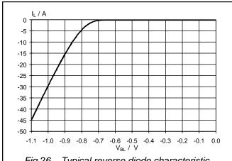
Fig.26. Typical reverse diode characteristic.  $I_L = f(V_{BL})$ ; conditions  $V_{IG} = 0$  V,  $T_j = 25$  °C
