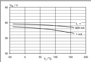
Fig.23. Typical battery to load clamping voltage.  $V_{\rm BL} = f(T_{\rm j})$ ; parameter  $I_{\rm L}$ ; condition  $I_{\rm G} = 10 {\rm mA}$
