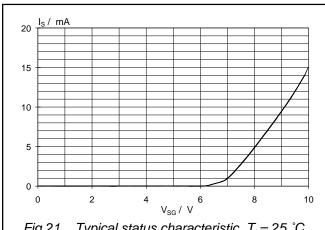
Fig.21. Typical status characteristic,  $T_j = 25$  °C.  $I_S = f(V_{SG})$ ; conditions  $V_{IG} = V_{BG} = 0V$
