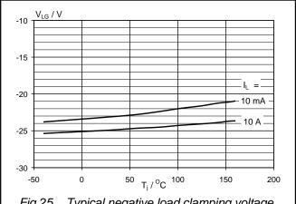
Fig.25. Typical negative load clamping voltage.  $V_{LG} = f(T_j)$ ; parameter  $I_L$ ; condition  $V_{IG} = 0$ V
