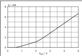
Fig. 19. Typical status low characteristic,  $T_i = 25$  °C.  $I_S = f(V_{SG})$ ; conditions  $V_{IG} = 5V$ ,  $V_{BG} = 13V$ ,  $I_L = 0A$
