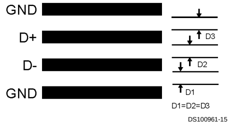
FIGURE 6. Recommended Diode Trace Layout
