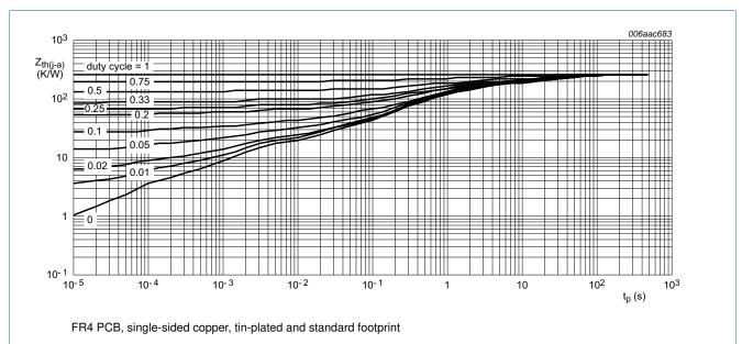
Fig 2. Transient thermal impedance from junction to ambient as a function of pulse duration for; typical values
