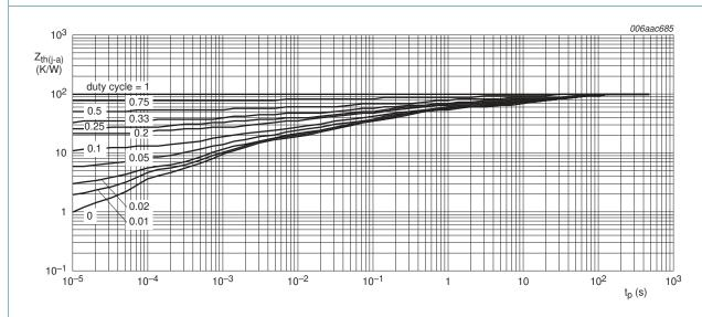
FR4 PCB, single-sided copper, tin-plated and mounting pad for collector 6 cm<sup>2</sup>
