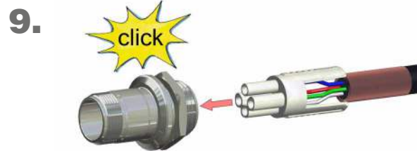
9. Put insulation part (2) into housing (3) 🗨 Pay attention to notches.
