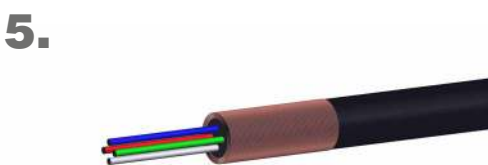
5. Remove any filling elements from cable
