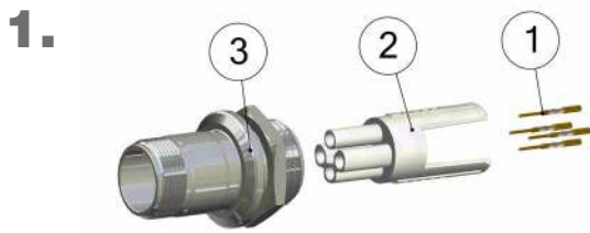
1. Part as delivered contacts (1), insulation part (2), housing (3)
