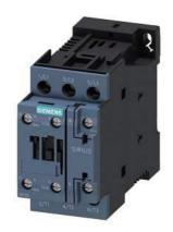
power contactor, AC-3e/AC-3, 32 A, 15 kW / 400 V, 3-pole, 24 V DC, with plugged-in varistor, auxiliary contacts: 1 NO + 1 NC, screw terminal, size: S0  $\,$
