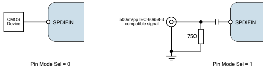
Figure 14 SPDIFIN Example External Connections
