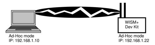
Since the WISM+ has been configured and reset into Ad-Hoc mode, now we have to go to the PC side and configure its Ad-Hoc wireless connection.
