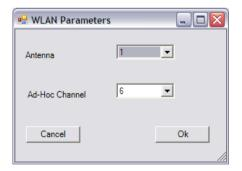
By pulling down the Antenna selection box, you can select U.FL port #1, U.FL port #2 or the diversity option in which two antennae MUST be used.
