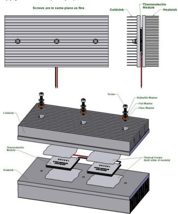
NOTE: Graphite pads may also be used as a thermal interface and require a higher clamping pressure depending on system set up. Please check thermal interface manufacturer instructions.
