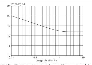
Fig.5. Maximum permissible repetitive rms on-state current  $I_{T(RMS)}$ , versus surge duration, for sinusoidal currents, f = 50 Hz;  $T_{mb} \le 100$  °C.
