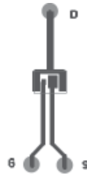
③ Mounted on minimum footprint full size board with metalized back and with small clip heatsink (still air)
