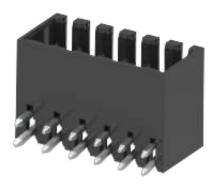
PCB connector Rated current: 7 A Rated voltage: 150 V Pitch: 3.5 mm Mounting: Reflow soldering
