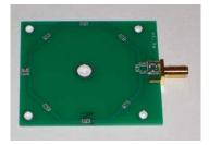
This antenna is well suited for reading the near-field loop incorporated into many Gen-2 tags. This antenna requires a coax cable with a reverse-polarity SMA connector at one end for connection to the DLP-RFID-UHF1B reader. A 3-foot coax cable is provided with each DLP-RFID-UHF1B reader purchased from DLP Design.
