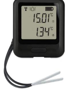
The sensor is IEEE 802.11bgn\* (2.4GHz) compliant, supports WEP, WPA/WPA2 encryption and enterprise networks (PEAP, TTLS, FAST).
