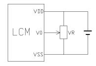
VDD-V0: LCD Driving voltage
