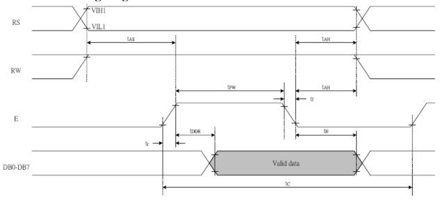
Write cycle (Ta=25°C, VDD=5.0V)
