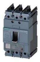
circuit breaker 3VA5 UL frame 125 breaking capacity class S 25kA @ 480V 3-pole, line protection TM230, FTAM, In=50A overload protection Ir=50A fixed short-circuit protection Ii=5...10 x In UL 489 SB (naval), 50° C without connection
