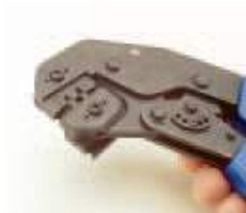
1. Cycle the CCT - SLE / SLC hand tool to the open position.
