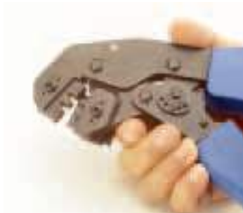
2. While pressing upward on the locator spring, insert the contact with tails upward completely into the locator.
