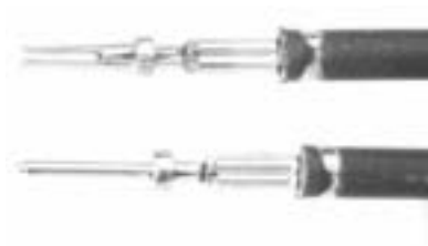
8. Note that there are no unterminated wire strands, and that some strand ends can be seen at the forward edge of the crimp. Also note the insulation is gripped by the smaller secondary crimp. Distortion is at a minimum, both axially and laterally - no sharp edges.
