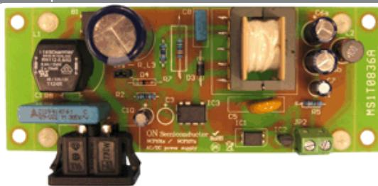
Unlike other monolithic solutions, the NCP1072/5 is quiet by nature: during nominal load operation, the part switches at one of the available frequencies (65, 100 or 130 kHz). When the output power demand diminishes, the IC automatically enters frequency foldback mode and provides excellent efficiency at light loads. When the power demand reduces further, it enters into a skip mode to reduce the standby consumption down to a no load condition.
