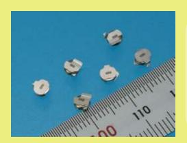
XH311HG is a coin type capacitor (D: 3.8mm / H: 1.1mm), with a unique quality of large current discharge, ranging from 3.3V to 0V. It is Pb-free reflowable with a high temperature heat resistance (Peak temparature of 260°C).
